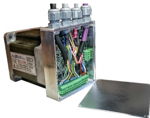
Fig. 1 FD2 applied on NEMA 34 stepper motor.
